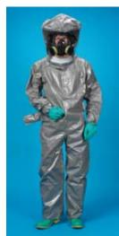
Encapsulated suit, rear entry, flat back, 48" zipper, storm flap, 20 mil PVC face shield, elastic wrists, 1 exhaust port with shroud, air tube inlet, attached sock boots with boot flap.
