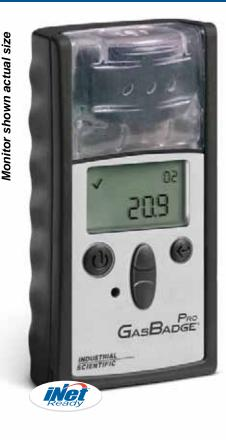
uilt to Industrial Scientific's highest quality and reliability standards, GasBadge® Pro provides a lifetime of gas hazard protection with more features than any other single gas monitor available. Interchangeable "smart" sensors enable the GasBadge Pro to be quickly adapted to monitor unsafe levels of oxygen or any one of the following toxic gases: carbon monoxide, hydrogen sulfide, nitrogen dioxide, sulfur dioxide, chlorine, chlorine dioxide, phosphine, ammonia, hydrogen cyanide and hydrogen.
