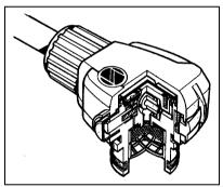
The DV operates in conjunction with the facemask spring-loaded exhale valve to maintain a positive pressure within the facemask.
