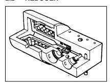
The pressure reducer operates on a selfregulating, spring-loaded piston principle that is completely automatic in operation and requires no adjustment.
