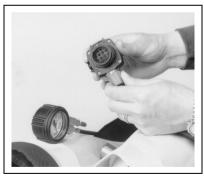
1. Open bypass knob slightly to vent air from system. Check that the whistle sounds clearly at between 63 and 73 bar. When all air has been released, close bypass.
