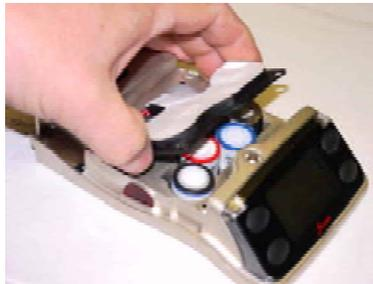
4.) Remove and replace the plug-in sensor.
