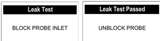
**Scout with Hand Aspirator:** To test for leaks, squeeze the Aspirator bulb until fully deflated, and hold deflated, then place your finger over the end of the Probe and release the bulb. The bulb will remain deflated if no leaks are found. Remove your finger from the end of the probe and the aspirator bulb will inflate.
