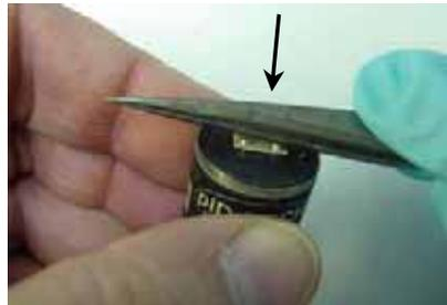
Reinstall the Cap and Filter Assembly by pushing it down on the sensor housing uniformly until it snaps into place. Make sure that the hole in the Cap and Filter Assembly is aligned over the holes in the metallized Detector Element (Figure 17).
