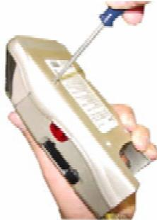
3.) Lift the rubber sensor gasket assembly away from the sensor chamber. Inspect the sensor filter material located on top of the rubber sensor gasket replace the sensor gasket assembly if dirty or deformed.
