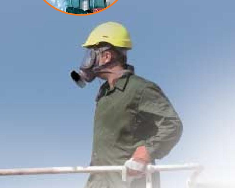
The Sari NR is a natural rubber face mask with a wide-vision panoramic visor and a central, front fitting filter port. In common with all the full face masks in the Scott range, it utilises airflow management to prevent visor misting and to ensure CO<sub>2</sub> is flushed rapidly and efficiently, greatly enhancing acceptance and reducing fatigue.
