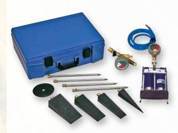
Sealing wedges and sealing cones are new additions to the Sava sealing products line. Sealing wedges and cones are used for quick sealing of cracks or slot shaped punctures on ground storage tanks or tankers on trucks and railcars. Three different size wedge shaped plugs are included, which can be used for sealing cracks (15 - 60 mm). One cone shaped plug is included, which can be used for sealing holes 30 - 90 mm. diameter.
