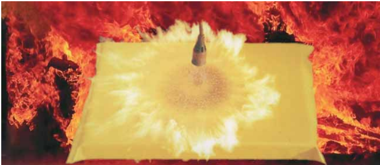
The cover of the mattress and pillow withstands gas burner at 900 degrees Celsius.
