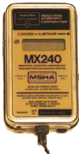
Early O 2 and Methane two-gas instrument
