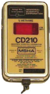
Early Methonometer ends flame safety lamp
